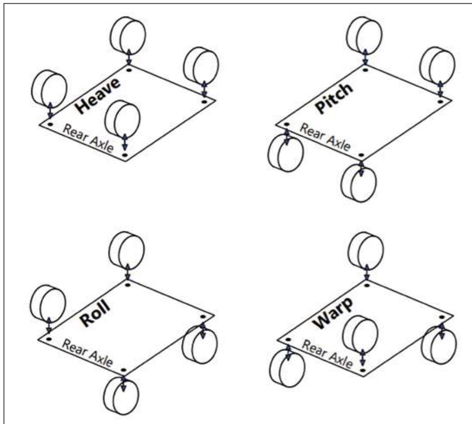
Figure 1: The four different modes of suspension motion
