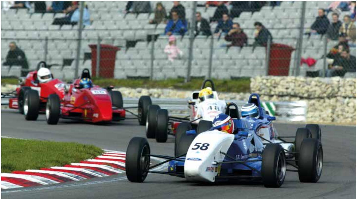
When a racecar has low or no downforce, as is the case with these Formula Fords, dampers should be selected to minimise the TLV in order to maximise the mechanical grip
