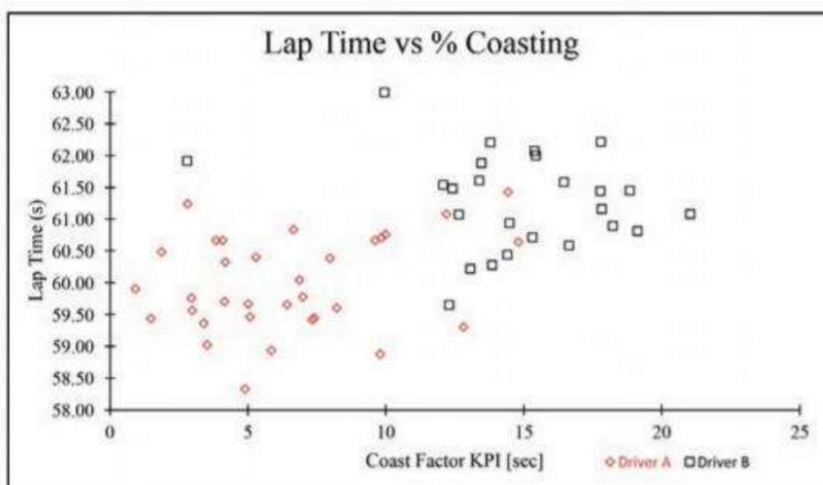
**Figure 4: This shows the lap times relative to the time each driver spends coasting**
