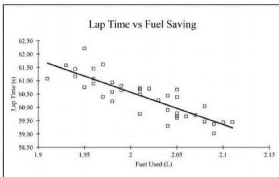
**Figure 7: Comparison of lap time vs fuel used. This is very useful for devising strategies**
