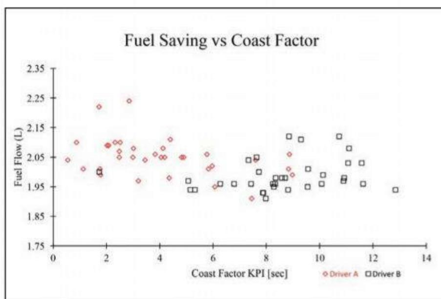
**Figure 6: The correlation of coast factor to the fuel savings for each lap during a stint**
