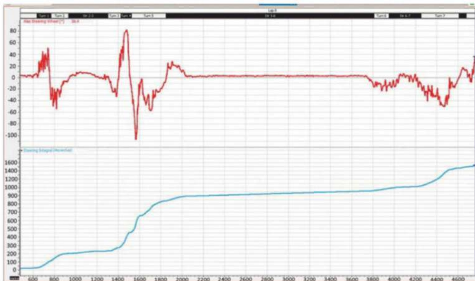
Figure 3: Red is steering wheel angle for a lap while blue is the steering wheel angle integral obtained from Table 1
