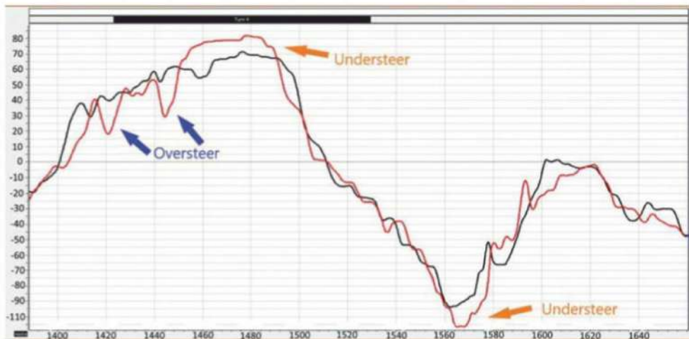
Figure 1: Steering wheel angle with reference lap (in black) and fastest lap (in red) with handling states indicated
