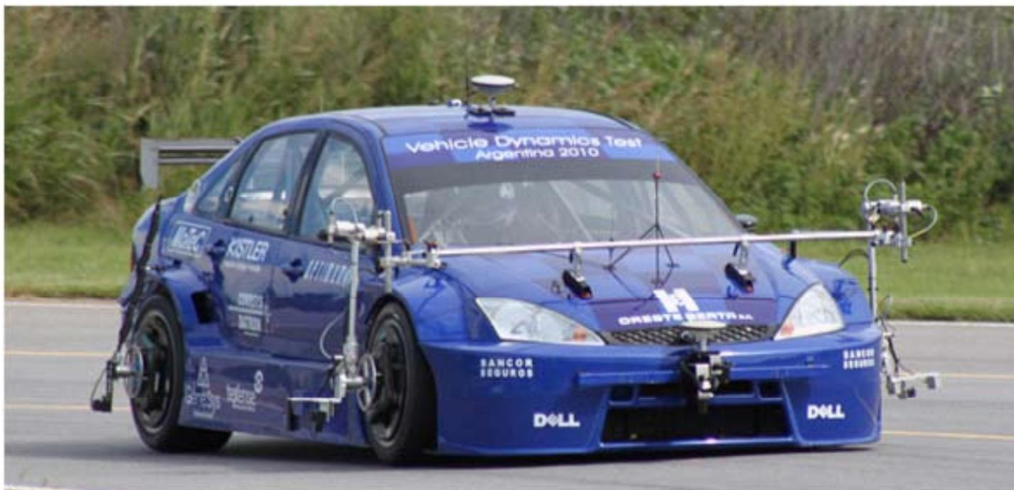
Figure 1: The vehicle and sensors used for the testing. This car was built for the Argentinean TC2000 racing series.
