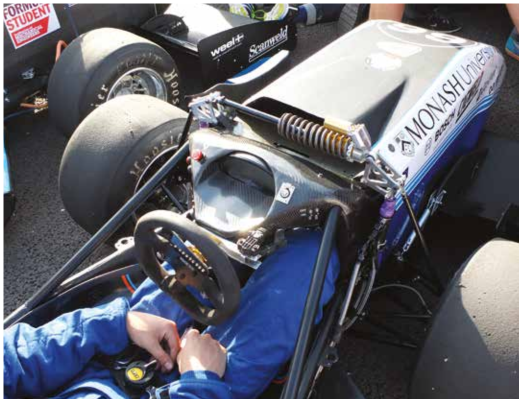
Cockpit ergonomics are a crucial part of the Formula Student design process. Your driver must be able to feel and control the racecar properly and it is important that no part of the chassis restricts movement
