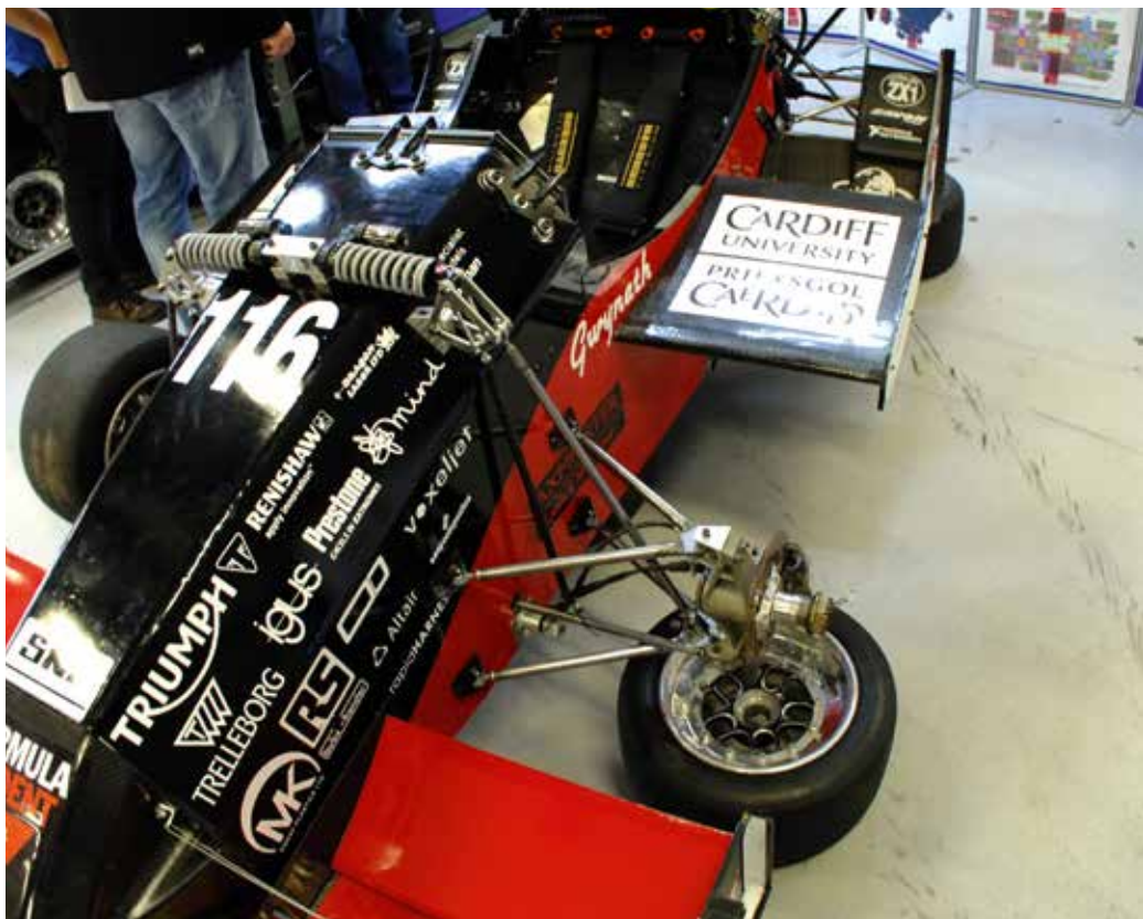
It's worth including some adjustability in suspension pick up points in both your upright and your chassis design. A difference of just a few millimetres can sometimes reward you with a major performance gain
