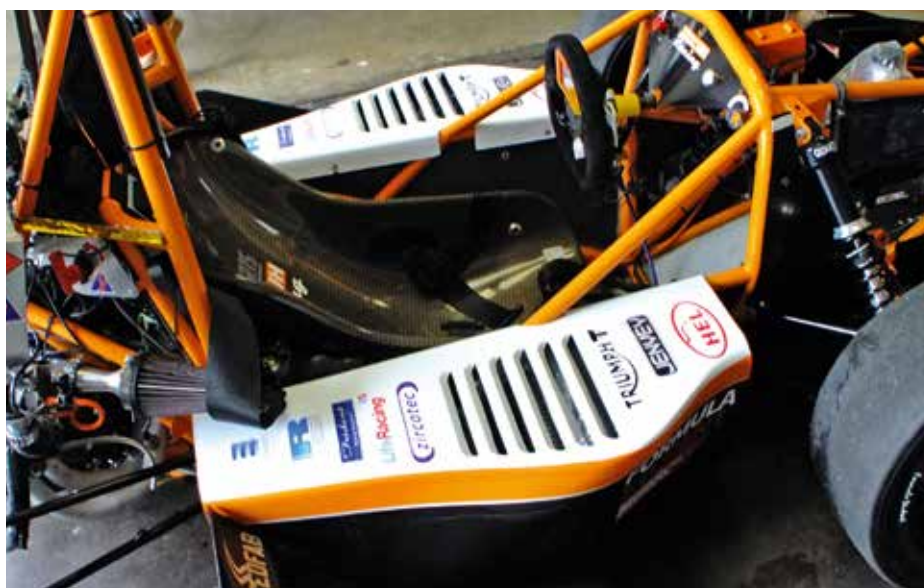
Bodywork pieces such as sidepods and engine covers need to be removed and then replaced within 30 seconds. Similarly, any toe, camber or ride height adjustment should not take more than two minutes
