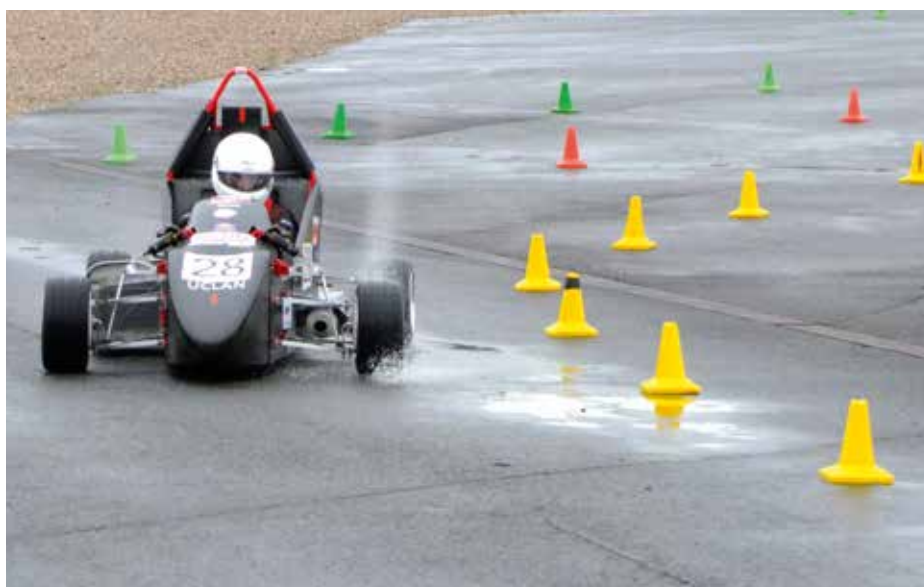
Competing in the wet is about more than simply considering the reduced grip – for instance, brake fluid is hygroscopic and so this needs to be flushed out and replaced after the racecar is taken out in the rain
