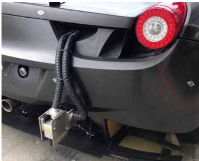
Here OptimumG has installed one of its slip angle sensors on the back of a GT car
