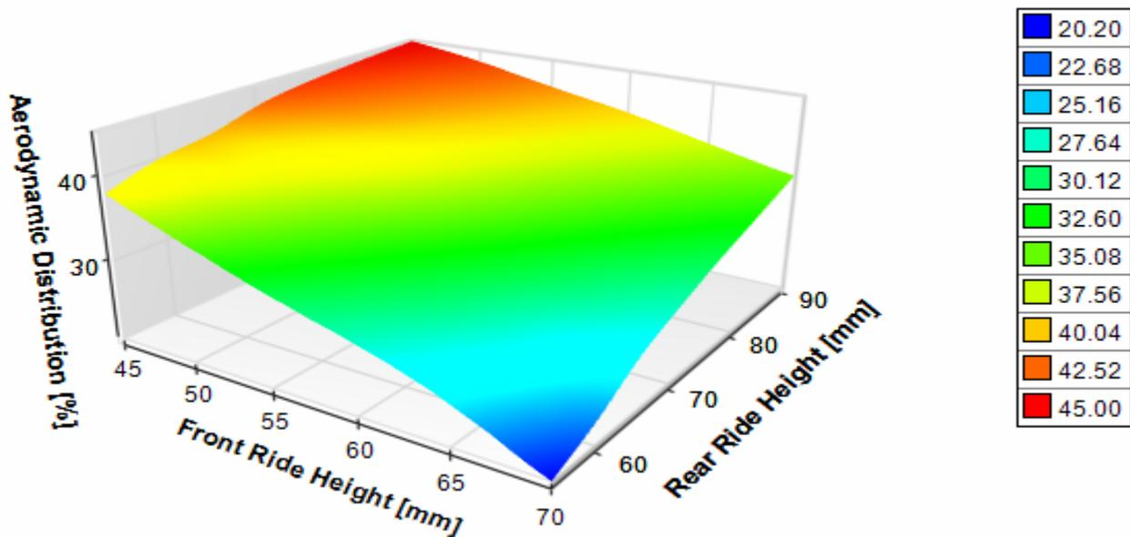
**The 3D graphing feature within OptimumDynamics helps visualize the change in aerodynamic distribution**
