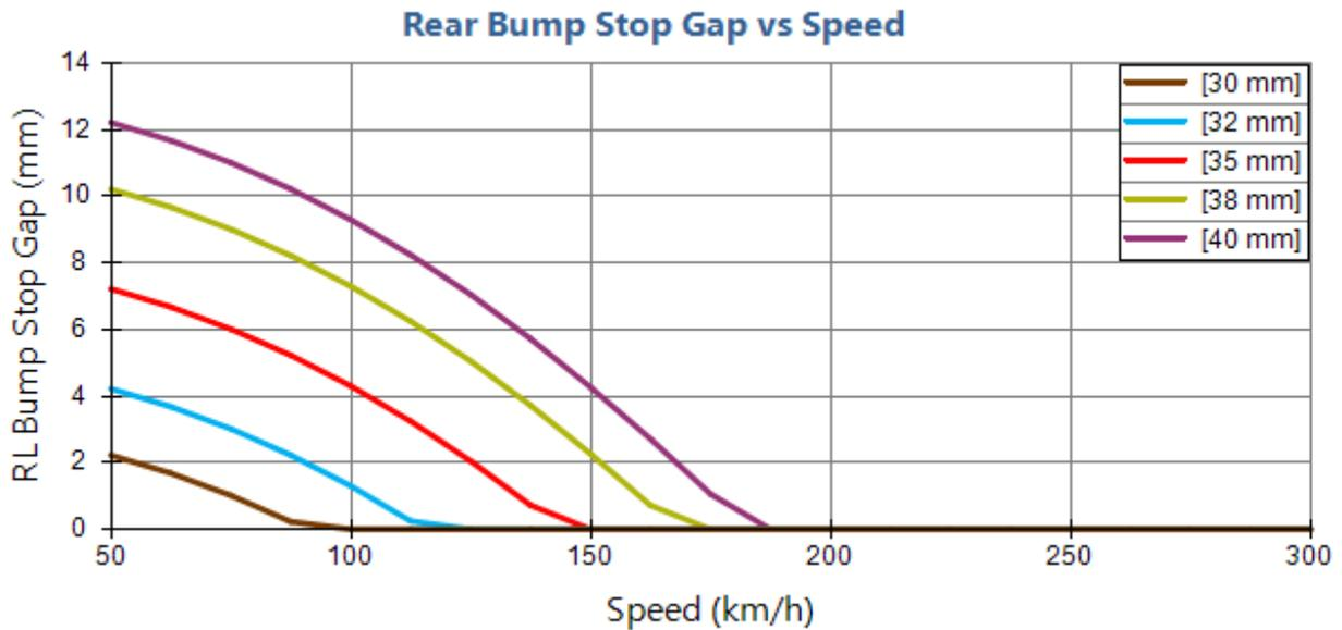
**BELOW** - We now proceed to create a plot of full droop bump stop gap and the speed at engagement. In this plot we can see the non-linear relationship between these two
