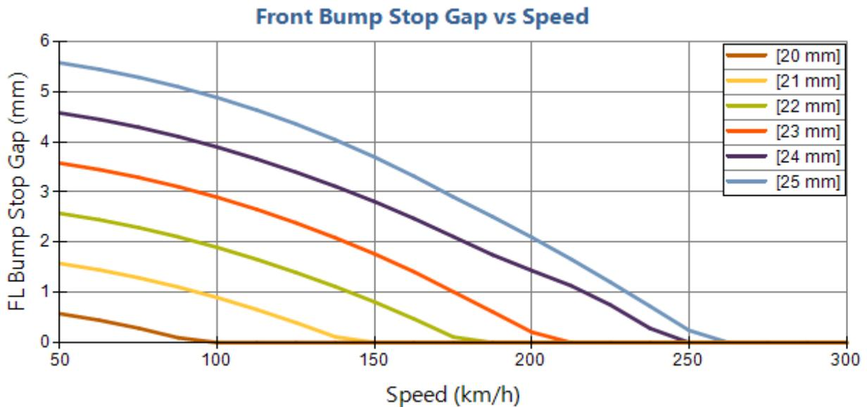
From these results we can create a chart relating the full droop bump stop gap to the vehicle speed at which it engages (*speed at engagement*).
