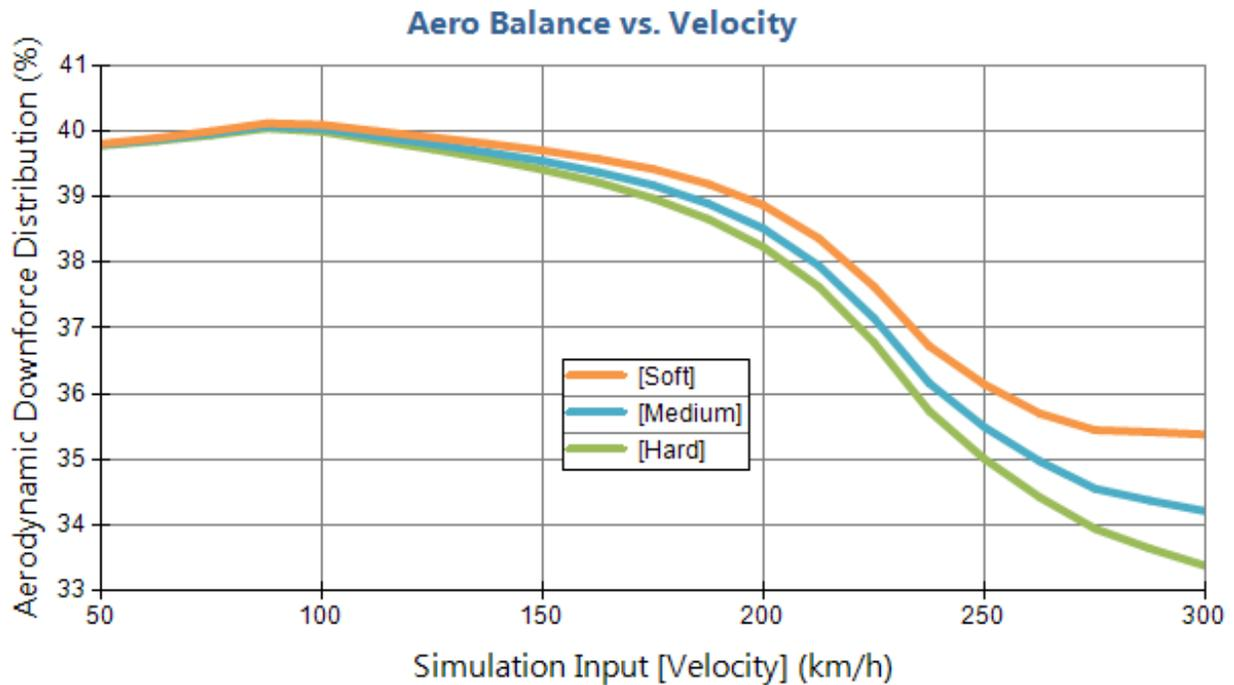
**ANALYSIS** - One of key findings from the plot is the non-linearity in the aerodynamic distribution with speed. We are able to see this effect thanks to the full vehicle kinematics model and the ride height sensitive aero maps used in
