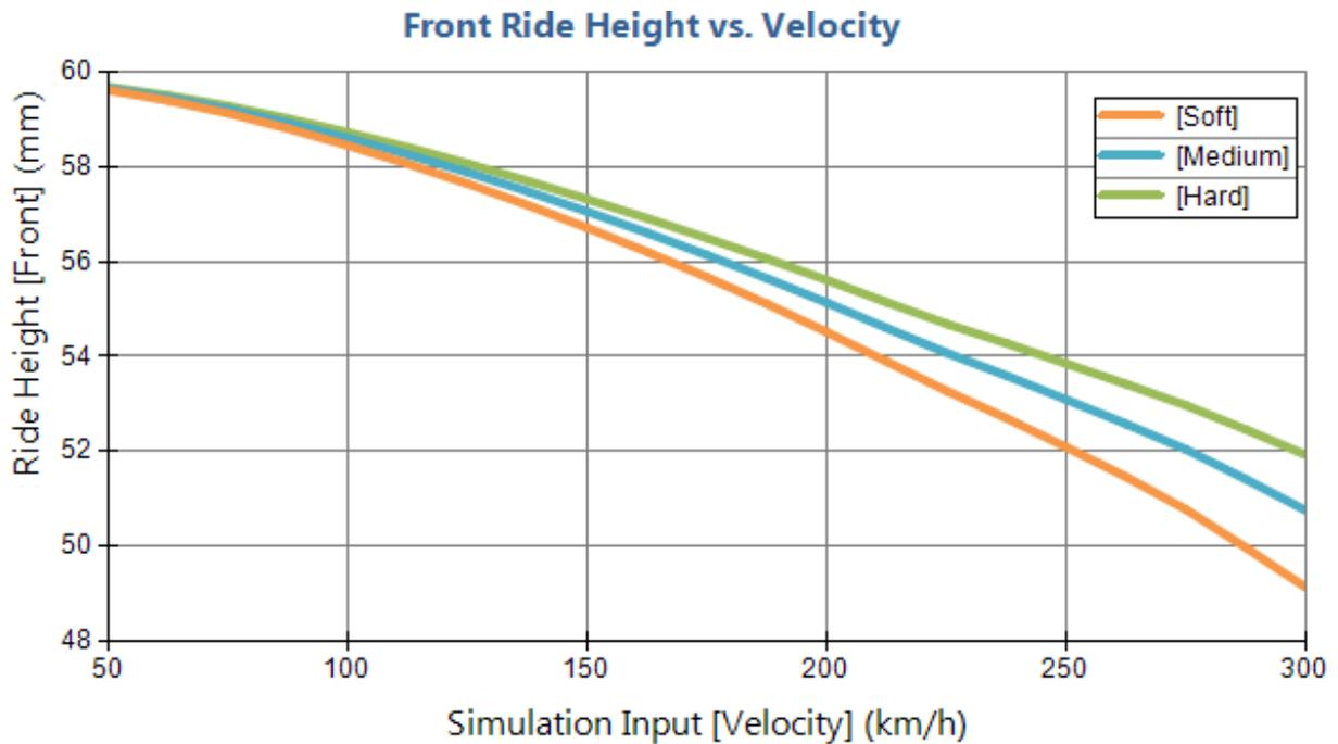
Using these results we can determine the influence of spring changes on aerodynamic distribution at different speeds. At one of the tracks, the average cornering speed of this GT racecar is between 160 and 200km/h with a top speed of 240km/h. Presented below is a table summarizing the simulation results at these vehicle speeds.
