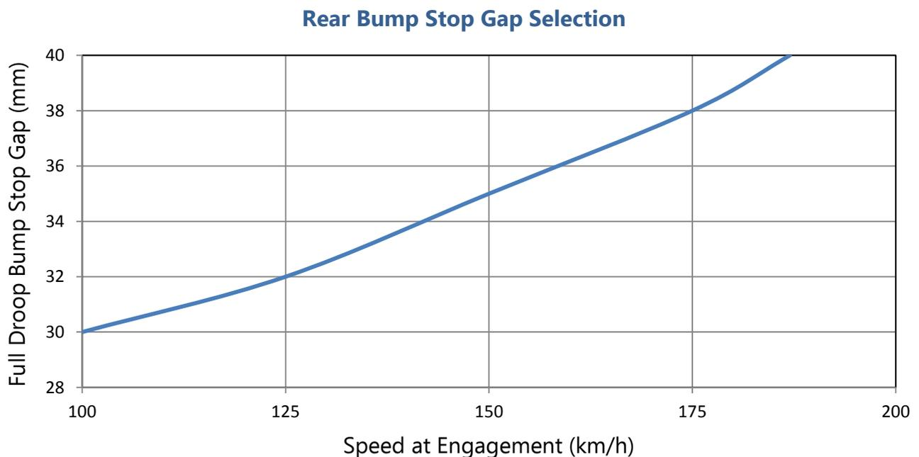
Using these results we can now determine our full droop bump stop gap depending on the vehicle speed at which they should engage. Let's say that we would like the vehicle to have its rear bump stop engaged
